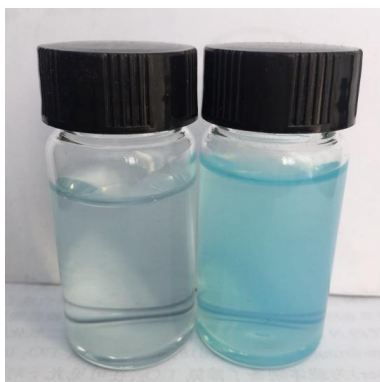
Figure 6. Photographs showing the enhanced degradation of methylene blue after treatment of CQDs/P25 (left) as compared with P25 (right).
