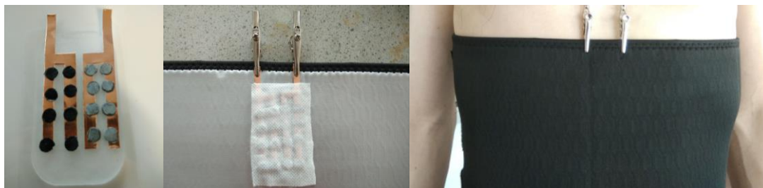
Figure 6.6 (a) Left: DUFC using 10% Ni-doped Cu@Cu-Zn as anode, C/CQD as cathode and hydrogel as flexible substrate (b) Middle: A piece of gauze covers the side with electrode discs of DUFC, and DUFC is fixed on the sweat belt. (c) Right: Experimenter wearing the sweat belt with DUFC
