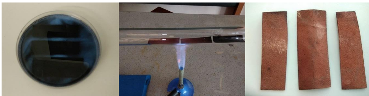
Figure 2.1 (a) Left: 3 copper foam strips immerse in the alkaline K_2S_2O_8 solution. (b) Middle: oxidized copper foam strips under chemical reduction by flowing hot town gas. (c) Right: reduced copper foam strips with nanostructure.
