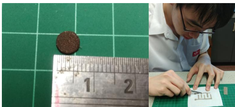
Figure 4.2 (a) Left: electrode discs with 6 mm diameter were punched (b) Right: fixing the metal strip (copper or nickel) to give a circuit
