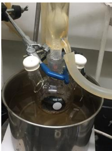
Figure 7. Synthesis of the iridium chloride bridge dimer
