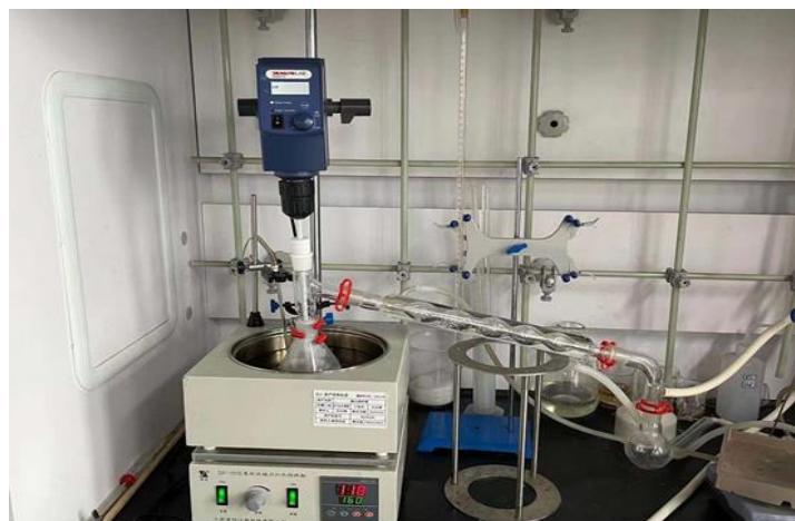
Figure 2.6 A round bottom flask with magnetic stirring and distillation head The conversion rate of DMT can be calculated by the following formula.
