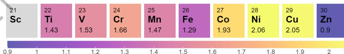
**Figure 6.** The energy barriers (eV) of methane oxidative dehydrogenation on 3d-MN<sub>4</sub>-G
