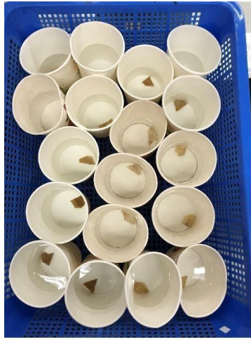
Measuring the percentage of water absorbed by different samples of kombuchas (lemon skins & orange skins)
