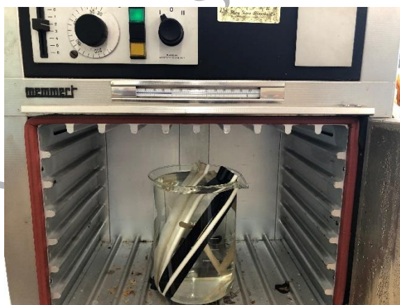
Testing heat endurance of straws (in 95°C hot distilled water in an oven at 50°C for 30mins)
