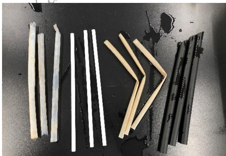
Roasted kombucha straws bio-degradable paper straws PLA straws plastic straws
