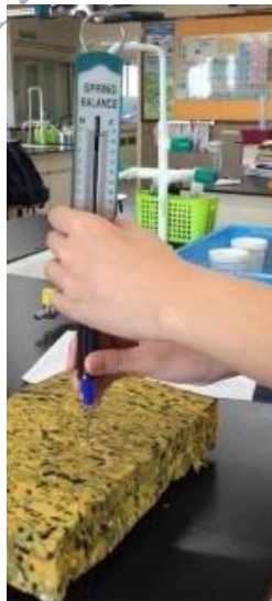
Measuring the force applied to punch through samples of roasted kombuchas
