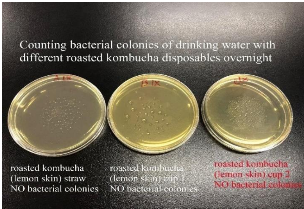
Fig.3.6.3 Counting bacterial colonies of drinking water kept in roasted kombucha straw (lemon skins)(left) and soaked with kombucha cups(lemon skins)(middle & right) overnight
